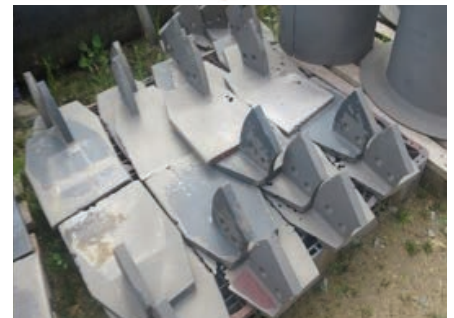
Berg design with coating: This is after 18 months of use in the feed end compartments – client will still get another 9 months out of these in the discharge end compartments.
